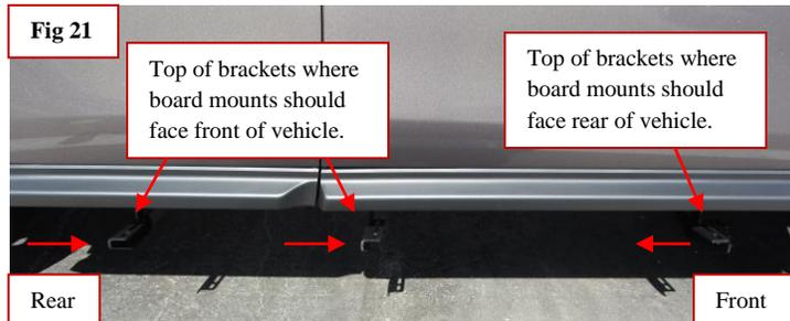
**Step 13:** Now install running boards on the brackets. Obtain the bracket to board bolt pack. Take out the provided 5/16" \* 3/4" bolts. Slide the head of the bolts down the channels on the underside of the board.
