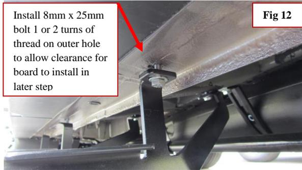
**Step 6:** This is the front passenger bracket installed. Bracket is shown fully tightened but should be installed loose as indicated Step 5 (Fig 12)
