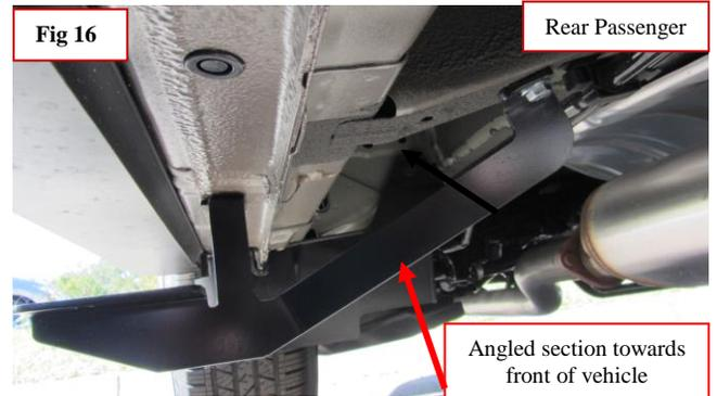
**Step 9:** The front driver bracket will install just like passenger in the 2nd black plug. Remember to install loose as indicated Step 5 (Fig 12)
