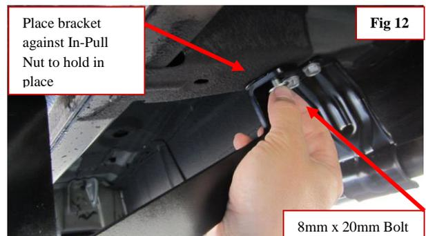
**Step 5:** Install 8mm x 25mm fasteners in all holes where you've removed the black plug. You will only install the bolt 1 to 1 ½ turns, just enough to hold bracket in place. This will be an important step to allow board to be installed on the brackets with the small amount of room available
