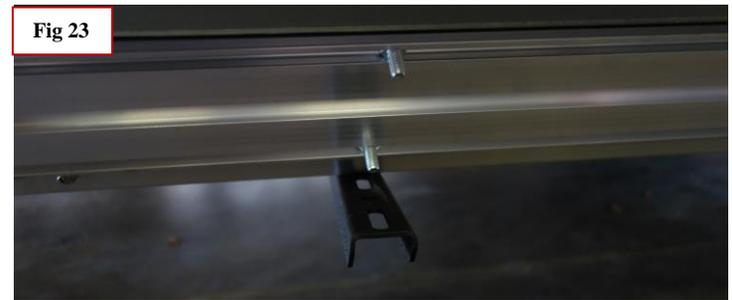
Now loosely tighten outer bracket bolts left slightly threaded from Step 5 (**Fig 12**). Adjust the board in or out, right or left to meet your needs. Once the boards are in place to your liking, tighten all fasteners on the brackets then the boards. Front and rear brackets should be adjusted all the way out away from the vehicle for best fit. This will complete your installation. Enjoy!
