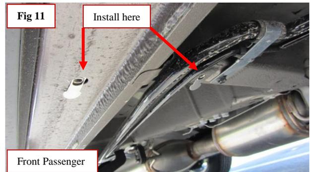
**Step 4:** The easiest way to install the brackets is to place bracket against In-Pull Nut holding it in place with the slot lined up with the hole in the In-Pull Nut. Now use the provided 8mm x 20mm bolt & washer to loosely secure inner hole in bracket.
