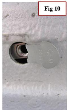
**Step 3:** Starting on passenger front. Remove 2nd black plug and install In-Pull nuts as shown (Fig 11)
