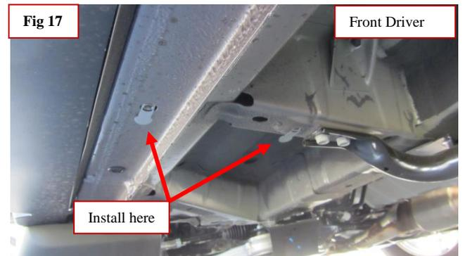
**Step 10:** The middle driver bracket will install just like passenger in the 4th black plug. The back of this bracket will install using an In-Pull Nut not a factory bolt. Remember to install loose as indicated Step 5 (Fig 12)
