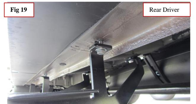
**Step 12:** Rear splash guard will need to be removed or cut to have boards fit properly on vehicle.
