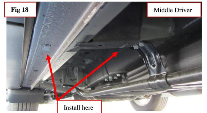
**Step 11:** The rear driver bracket will install just like passenger in the 6th black plug. Remember to install loose as indicated Step 5 (Fig 12)
