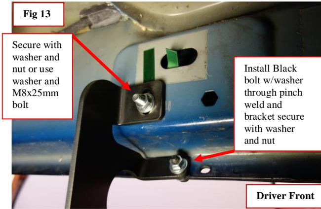
**Step 7:** Middle Driver will install the same as the front it will use (2) bolts in the pinch weld. Snug all fasteners to hold bracket but do not tighten.
