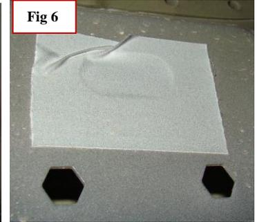
**Step 3:** We need to remove the factory tape at each location. Peel it off and keep it clean. It can be put back to its original place after the bolt plate is installed.
