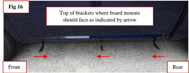
**Step 9:** Now install running boards on the brackets. Obtain the bracket to board bolt pack. Take out the provided 5/16" \* 3/4" bolts. Slide the head of the bolts down the channels on the underside of the board.
