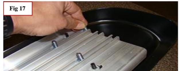
**Step 14:** Place the board on the installed mounting brackets. Align the bolts with the slots on the brackets and drop them into place. Next thread the provided 5/16" flange nuts onto the bolts to hold the board and leave loose. Adjust the board in or out, right or left to meet your needs. Once the boards are in place to your liking, tighten all fasteners on the brackets. Front and rear first and then the center brackets finally the boards. This will complete your installation. Enjoy!
