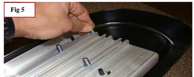
**Step 6:** Place the board on the installed mounting brackets. Align the bolts with the holes on the brackets and drop them into place. Next thread the provided 5/16" flange nuts onto the bolts. Do not tighten. Adjust the board in or out, right or left to meet your needs. Once the boards are in place to your liking, tighten all fasteners on the boards and brackets. This will complete your installation. Enjoy!
