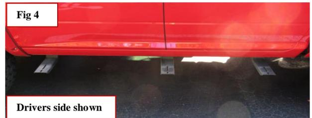
**Step 5:** Now install running boards on brackets. You may have different boards than shown. However, they will have the same type of mounting unless additional installation instructions are provided. Obtain the bracket to board bolt pack. Take out the provided 5/16" x 3/4" bolts. Slide the head of the bolts down the channels on the underside of the board.
