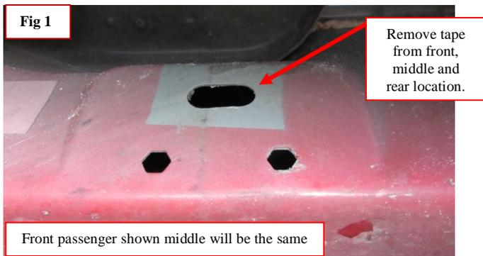
**Step 2:** Start by installing the double studded bolt plate through the bigger slot with the small stud coming through the hex hole and the longer stud through the big oval hole (**Fig 2**). Place plastic bolt retainer not shown over small stud in hex hole to stop bolt plate from falling into open cavity. It can be installed on threads by turning just like a nut. Driver side will use opposing hex hole for small stud.
