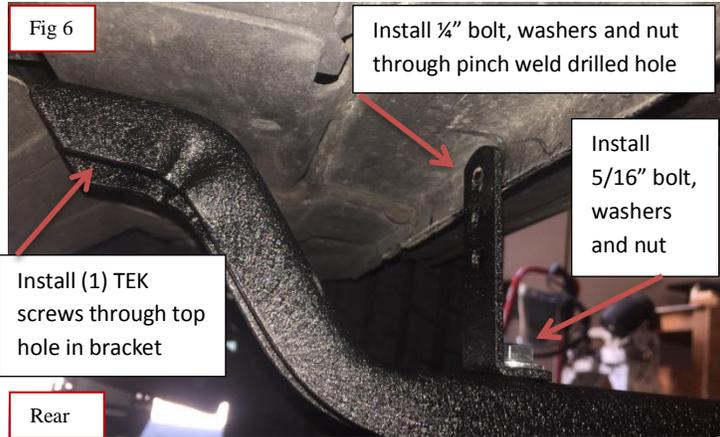
**Step 7:** When installing TEK screw in rear bracket in Step 8. Make sure bracket is protruding out from vehicle even with front, front middle & middle rear brackets.
