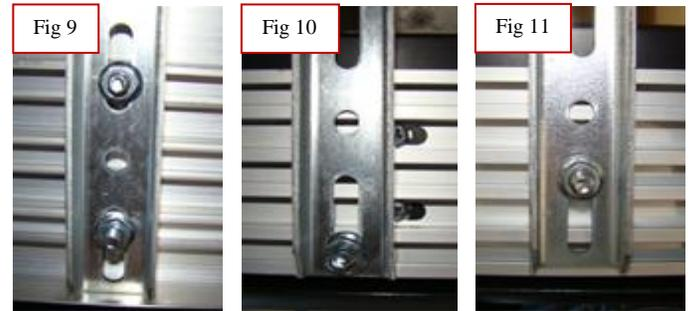
**Step 12:** Adjust board to center on cab front to back and adjust in and out for desired step area. Tighten outside brackets first then inside brackets accordingly. Fully tighten all brackets.
