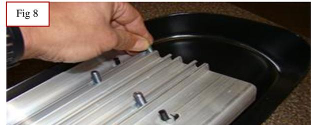
**Step 11:** There are several configurations to mount the boards to the brackets. We have provided some suggestions in the figures above. These changes allow you to adjust the board in or out according to your step preference. All are correct.
