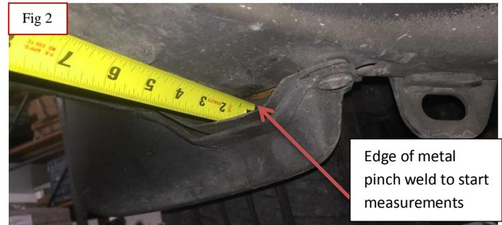
**Step 3:** Drill 1/4" holes in all four marked locations in pinch weld. **Note:** Drill each hole so that is center top to bottom on the pinch weld. Reference locations ( Fig 3,4,5 & 6)
