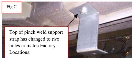
**Step 5:** Attach Front bracket to pinch weld support strap in location 1 using a hex head bolt, washer and serrated flange nut. Leave loose at this time.
