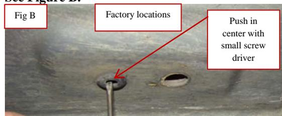
**Step 4:** Install Pinch Weld Support Straps in factory locations. Remember the rear location, the pinch weld support strap will be at a different offset angle than the rest of the support straps. Use two **8mm** bolts in locations 1, 2 and 3. See Figure C. In rear location use one **8mm** bolt. Tighten the bolts at this time.
