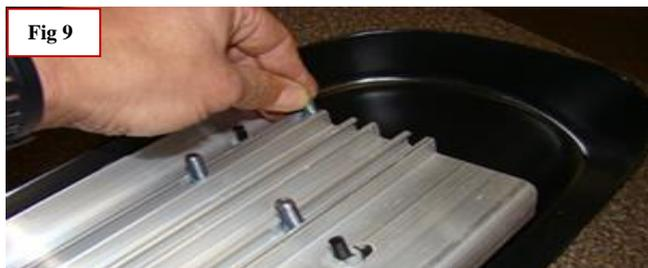
**Step 8:** Place the board on the installed mounting brackets. Align the bolts with the holes on the brackets and drop them into place. Next thread the provided 5/16" flange nuts loosely onto the bolts to secure brackets to the board (Fig 10)
