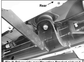
(Fig 2) Driver side rear Mounting Bracket pictured
