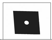
(Fig 2) Plastic Insulation Washer
