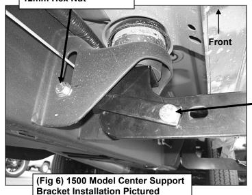
12mm x 30mm Hex Bolt (2) 12mm Flat Washers 12mm Lock Washer 12mm Hex Nut NOTE: Support Brackets not required on 2011-12 25-3500 Models
