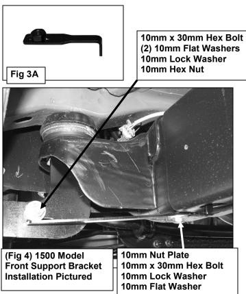
**IMPORTANT NOTE: 25-3500 Model Front Support Bracket Installation Pictured** Bend Support Bracket up by hand to meet the Front Mounting Bracket.
