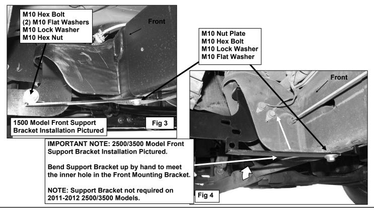
All 1500 and up to 2010 2500/3500 Models - Support Brackets not required on 2011 - 2012 2500/3500 Models:
