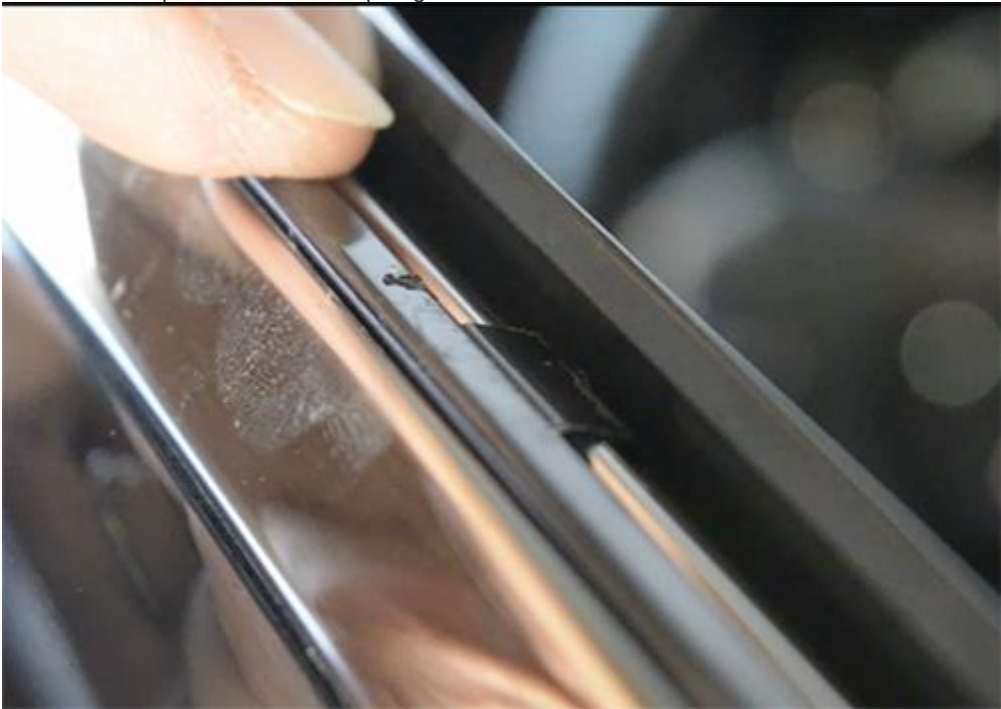
7. Mount the top brackets to the top edge of the door frame
