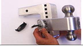
**STEP 3:** Once you have achieved the desired position along the <u>Drawbar</u>, insert the <u>Key Lock</u> <u>Assembly (D)</u> into the <u>180 Slider</u> and lock in place by turning the key.
