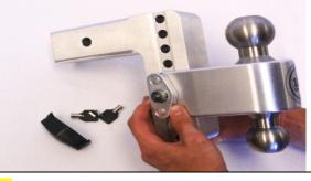
**STEP 4:** Pull on the <u>Key Lock Assembly</u> to ensure that it has engaged and place the <u>Dust Lock Cover (E)</u> over the lock. Do not operate without making sure the <u>Key Lock</u> <u>Assembly</u> is securely locked in place.
