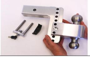
**STEP 1:** Ensure that the <u>180 Hitch Ball Pin (A)</u> is inserted fully into the <u>180 Slider (B)</u>. This pin should already be engaged and generally isn't supposed to be removed. Do not operate without <u>180 Hitch Ball Pin</u> in place.
