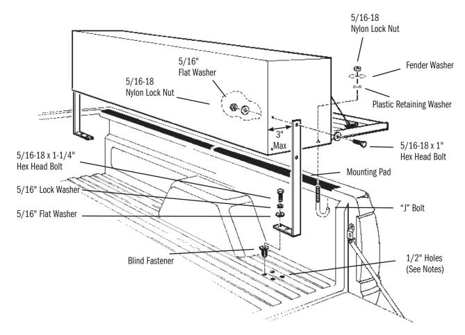
Place the mounting pads in position on top of the truck bed as shown in figure below. Tape the mounting pads to the truck bed in a few places to keep them from moving or falling off when installing the box.
