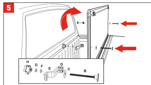
Fold back the cab panel and assemble the cab clamp (E)through the lifted panel. Start with the bolt (B) and rubber washer (C) through the top side of the panel. Followed by the cab clamp (E) with risers, then the steel washer (F), split washer (G), and finally the lock knob (H) through the underside. Repeat on the opposite side of the truck bed.
