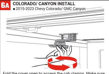
Fold the cover open to access the cab clamps. Make sure that the cab clamp is under the metal bed flange of the truck bed rail. Hand-tighten the knob. Repeat on the opposite side of the truck bed.
