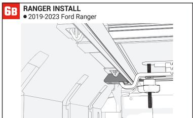
Position the spacer (O) under the truck bed rail and align it so the front clamp of the cover inserts into the slot of the spacer. Tighten the cab clamp to hold the spacer in place. Install one on both driver and passenger sides.
