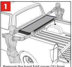
Remove the hard fold cover (A) from the box and place it on the cab end of the truck.
