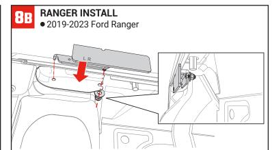
Align the Ranger rear bracket (P & Q) with the hole and slot at the tailgate end of the truck bed as shown. Install the washer (R) and nut (S) onto the threaded stud of the rear bracket (P & Q). Tighten the nut (S). Install one on each side of the truck bed, noting that there is a designated bracket for the driver (P) and passenger (Q) sides of the bed.
