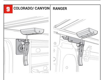
Clamps may need to be adjusted to accommodate different bed heights. Clamp height can be adjusted by turning the clamps clockwise or counter-clockwise to move the clamp higher or lower as needed.
