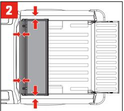
Set the cover (A) so the front seal is over the bulkhead and center the cover side to side.
