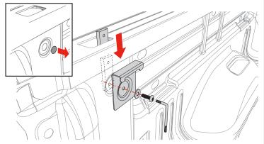
Remove the bed plug. Align the Colorado tail bracket (J) with the round dished area of the bed at the tailgate. Insert the slide block (K) into the stake pocket, align it with the screw (L) and washer (M). Tighten the screw (L) with the T-27 Torx key (N). Install one on each side of the truck.
