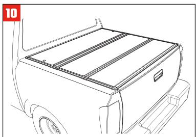
Close tailgate to check how the cover fits and adjust as needed. To make changes, loosen the cab clamps (E) and shift the cover into the appropriate spot, then retighten the cab clamps.
