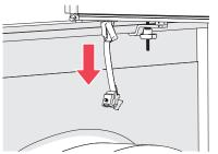
Pull the clamp down to tighten the knot. Make sure that the tether strap is tight around the cleat.
