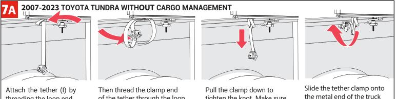
threading the loop end of the tether through the cleat under the cab panel. of the tether through the loop end of the tether.
