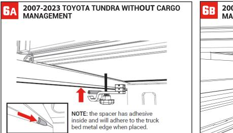
Fold the cover open to access the cab clamps. Install the bed flange edge spacer as shown. The spacer will slide onto the metal edge of the truck bed rail and align with the cover cab clamp. Hand tighten the knob. Repeat on the opposite side of the truck bed.
