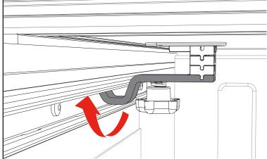
Fold the cover open to access the cab clamps (E). Hook the cab clamp (E) directly under the edge of the factory cargo rail. Tighten the lock knob (H). Repeat the steps on opposite sides of the bed. Snug firmly but do NOT overtighten. Reinsert any tie-down cleats in desired positions.
