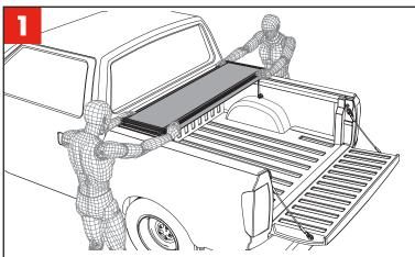
Remove the hard fold cover (A) from the box and place it on the cab end of the truck.
