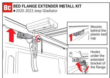
Fold the cover closed. Install the bed flange extender clamp (J) as shown. The clamp will slide onto the metal edge of the truck bed rail, it will be behind the plastic bed cap, align the clamp with the rear cover clamp. With the clamp positioned, hand-tighten the screws with the T27 Torx key (L). Swing the clamp down so that the jaw hooks under the extended bracket of the flange . Push the clamp handle toward the bed wall to lock it in place. Repeat on the opposite side of the bed.
