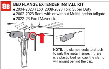
Fold the cover closed. Install the bed flange extender clamp (J) as shown. The clamp will slide onto the metal edge of the truck bed rail and align with the rear cover clamp. With the clamp positioned, hand-tighten the screws with the 5/32" hex key wrench (L). Swing the clamp down so that the jaw is under the edge of the bed flange extender. Push the clamp handle toward the bed wall to lock it in place. Repeat on the opposite side of the bed.
