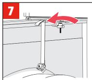
Attach the tether (I) by threading the loop end of the tether through the cleat under the cab panel.
