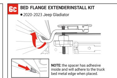
Fold the cover open to access the cab clamps. Install the bed flange edge spacer (K) as shown. The spacer will slide onto the metal edge of the truck bed rail and align with the cover cab clamp. Note that the metal flange is behind the plastic bed cap. Hand-tighten the knob. Repeat for the opposite side of the truck bed.
