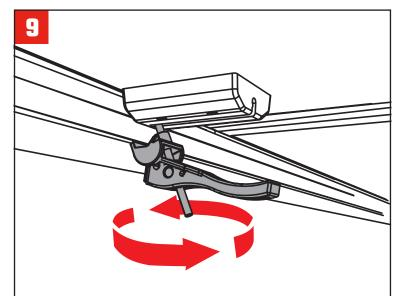
Clamps may need to be adjusted to accommodate different bed heights. Clamp height can be adjusted by turning the clamps clockwise or counter-clockwise to move the clamp higher or lower as needed.
