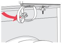
Then thread the clamp end of the tether through the loop end of the tether.
