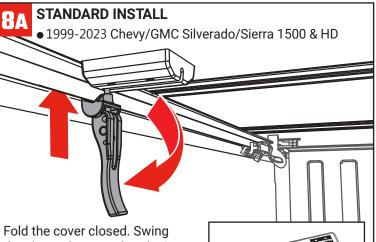
the clamp down so that the jaw is under the metal edge of the truck bed rail. Push the clamp handle toward the bed wall to lock it in place. Repeat on the opposite side of the bed.
