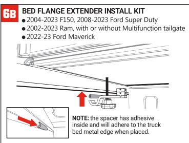
Fold the cover open to access the cab clamps. Install the bed flange edge spacer (K) as shown. The spacer will slide onto the metal edge of the truck bed rail and align with the cover cab clamp. Hand-tighten the knob. Repeat on the opposite side of the truck bed.
