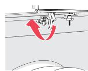
Slide the tether clamp onto the metal end of the truck bed flange and tighten the knob.
