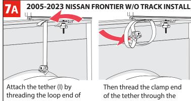
the tether through the cleat under the cab panel. loop end of the tether.
