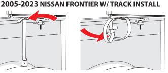
Then thread the clamp end of the tether through the loop end of tether.
