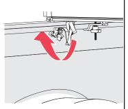
Slide the tether clamp onto the metal end of the truck bed flange and tighten the knob.
