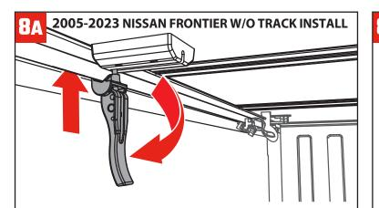
Fold the cover closed. Swing the clamp down so that the jaw is under the metal edge of the truck bed rail. Push the clamp handle toward the bed wall to lock it in place. Repeat on the opposite side of the bed.
