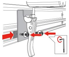
Fully close the cover. Slide the slide nut (N) into the end of the factory cargo rail, align the clamp bracket (O) with the tail clamp. Attach the clamp bracket (O) to the slide nut (N) using the screws (P) and washers (Q), tighten the screws (P) with the T27 Torx wrench (R). Swing the tail clamp down to lock it to the clamp bracket (O). Repeat the steps on both sides of the bed.
