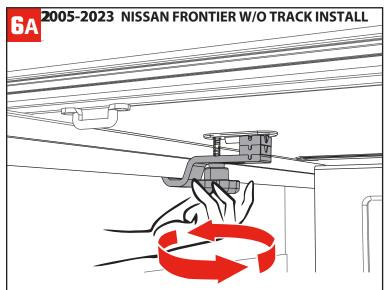
Fold the cover open to access the cab clamps. Make sure that the cab clamp is under the metal bed flange of the truck bed rail. Hand-tighten the knob. Repeat on the opposite side of the truck bed.
