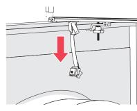
Pull the clamp down to tighten the knot. Make sure that the tether strap is tight around the cleat.
