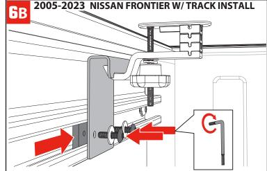
Fold the cover open to access the cab clamps (E). Insert the slide nut (N) into the end of the factory cargo rail, slide it to the front. Attach the front clamp bracket (O) to the slide nut (N) using the screws (P) and washers (Q). Align the clamp bracket (O) with the cab clamp (E) and tighten the screws (P) with the T27 Torx wrench (R). Tighten the lock knob (H). Repeat the steps on both sides of the bed. Snug firmly but do NOT overtighten. Reinsert any tie-down cleats in desired positions.
