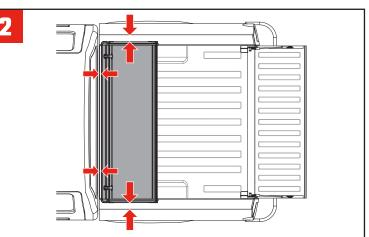
Set the cover (A) so the front seal is over the bulkhead and center the cover side to side.
