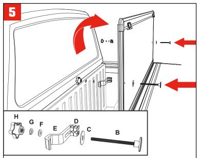
Fold back the cab panel and assemble the cab clamp (E) through the lifted panel. Start with the bolt (B) and rubber washer (C) through the top side of the panel. Followed by the cab clamp (E) with risers, then the steel washer (F), split washer (G), and finally the lock knob (H) through the underside. Repeat on the opposite side of the truck bed.
