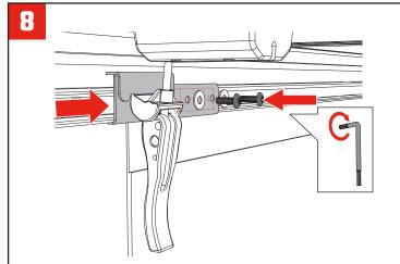
Fully close the cover. Slide the slide block (J) into the end of the factory cargo rail, align the clamp bracket (N) with the tail clamp. Attach the rear clamp brackets (R & S) to the slide block (J) using the screws (0) and washers (P), tighten the screws (O) with the T27 Torx wrench (Q). Swing the tail clamp down to lock it to the clamp bracket (N). Repeat the steps on both sides of the bed.
