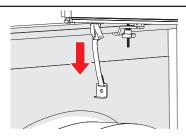
Pull the clamp down to tighten the knot. Make sure that the tether strap is tight around the cleat.
