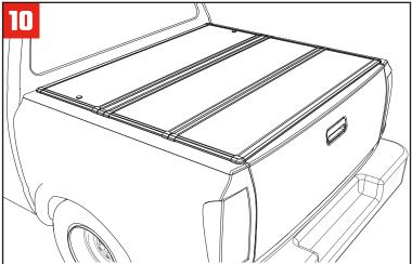
Close tailgate to check how cover fits and adjust as needed. To make changes, loosen the cab clamps (E) and shift the cover into the appropriate spot, then retighten the cab clamps.
