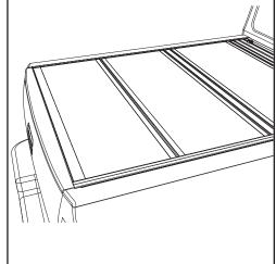
OPENING COVER: Lower the tailgate and pull the cable on either side. While pulling on the cable lift the panel up and towards the cab.
