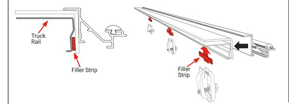
IMPORTANT: In order for the cover (C) to operate properly the side rails (A & B) MUST be square (90° angle) to the truck bed rails. This allows the rear latch to engage properly.
