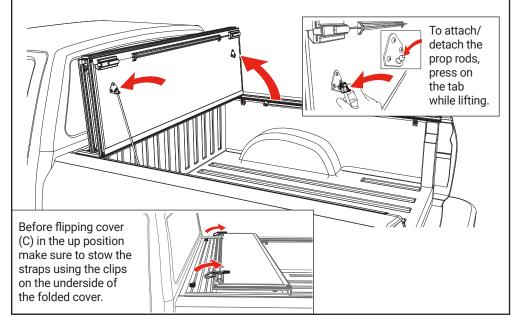
**CLOSING COVER:** To drive with the cover (C) closed, unhook the buckles and straps from the bulkhead. Stow the straps using the clips on the underside of the folded cover. Fold all panels towards the tailgate making sure that all latches are engaged.
