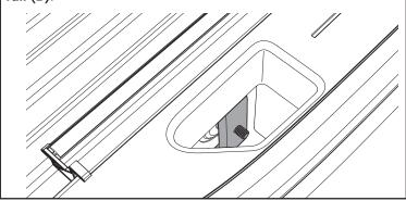
Position the buckle ends (H) with the open side facing the bed cover panel. Use a Phillips screwdriver to install the two buckles into the pre-drilled holes on the front header panel with the provided screws (I). **DO NOT use a** screw gun, securely tighten by hand only.
