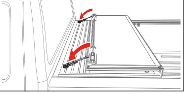
**FLIPPED UP POSITION:** Fold the cover (C) open and lift it until it's vertical towards your truck cab. Then release the prop rod that is attached to the side rail and clip it onto the ball stud on the underside of the cover.
