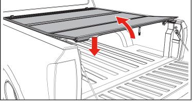
**FOLDED UP POSITION:** To drive with the cover (C) in the folded up position, use the straps and buckles provided with the cover. Attach the buckle at the bulkhead, then pull the strap to take up the slack and secure the cover.
