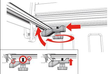
13 Unfold the cover (C) towards the tailgate. Then confirm each panel is centered side to side and front to back on the truck bed. If adjustments are needed, loosen the cover retainer clamps (F) and shift the cover (C) until positioned correctly. Retighten the cover retainer clamps once the desired fitment is reached. If adjustments to the slam latch are needed, see the directions on the next page.
