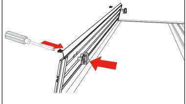
**12** Confirm the retainer clamps (F) are positioned around the side rails (A & B) correctly as shown below. Tighten the retainer clamps by turning them clockwise until the lock washer is secure.
