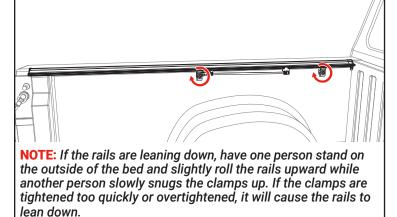
4 Place the passenger side rail (A) on the truck rail. Position the side rail flush with the top edge of your truck bed rail. The end of the side rail with the drain tube will go towards the cab of the truck. Repeat on the opposite side with the driver's side rail (B).
