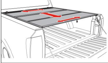
Power Tailgates: If your truck has a powered opening or closing tailgate ensure the tailgate functions properly with the cover closed and if needed adjust the cover towards the truck cab.
