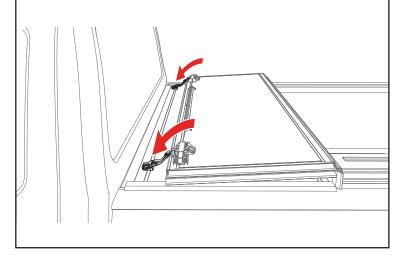
**CLOSING COVER:** To drive with the cover (A) closed, unhook the buckles and straps from the bulkhead. Stow the straps using the clips on the underside of the folded cover. Fold all panels towards the tailgate making sure that all latches are engaged.
