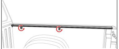
NOTE: If the rails are leaning down, have one person stand on the outside of the bed and slightly roll the rails upward while another person slowly snugs the clamps up. If the clamps are tightened too quickly or overtightened, it will cause the rails to lean down.
