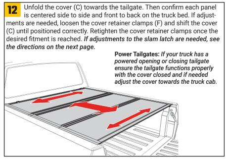
The rear edge of the cover (C) and tailgate seal should rest on top of the tailgate. You are ready to drive with your cover in the closed position.
