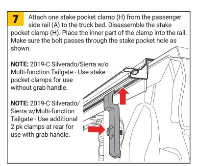
Place the outer part of the stake pocket clamp (H) into the stake pocket, up underneath the plastic bed cap, then secure to the bolt. Make sure the rail is level. Tighten all clamps to 10 ft/lbs of torque with a 1/2" wrench or socket. Caution: Do NOT overtighten! Install stake pocket covers (I) into stake pocket opening in the side rail toward cab and tail. Repeat steps 5-8 on the opposite side with the driver's side rail (B).
