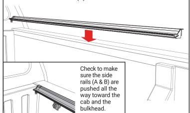
Attach two clamps (G) from the passenger side rail (A) to the truck bed. Place the front clamp 6-8 inches from the bulkhead. For the best cover, the side rails (A & B) should be level with the truck bed cap and not angled up or down.
