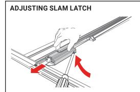
Use a screwdriver to partially pry open the tab on the latch housing. At the same time slide the housing away from the latch assembly.
