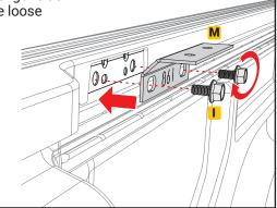
7 Installing Adaptor Rail: Install the adaptor rail driver side (D) and line up the front slotted holes with the holes in the front bracket using two M6 flange mounting bolts (I). Repeat on the opposite side using the passenger side adaptor rail (E). Do not tighten, leave loose at this time.
