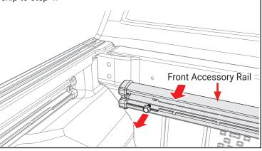
Installing Front Mounting Brackets: Use the driver side front mounting bracket (K) labeled with the letter "L". Locate the pre-bent tab on the front bracket and place in the upward most hole located towards the front corner of the bulkhead on both sides. Repeat on passenger side using the passenger side front mounting bracket (L) labeled with the letter "R".
