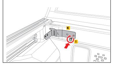
If you **DID** remove the front accessory rail, as mentioned in step 2, proceed to install the accessory rail over the front bracket (K) you just installed aligning the holes in both using one M6 flange mounting bolt (I) through both and into the bulkhead. Repeat on passenger side using the passenger side front mounting bracket (L) labeled with the letter "R". Then tighten bolts.
