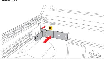
If you do not have a front accessory rail, as mentioned in step 2, proceed to install one M6 flange mounting bolt (I) into the front bracket (K) in the second slotted hole to the right as shown. Repeat on the passenger side using the passenger side front mounting bracket (L) labeled with the letter "R".
