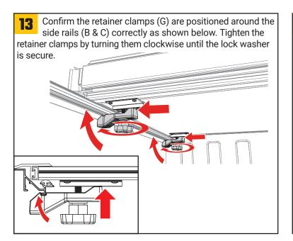
Unfold the cover (A) towards the tailgate. Then confirm each panel is centered side to side and front to back on the truck bed. If adjustments are needed, loosen the cover retainer clamps (G) and shift the cover (A) until positioned correctly. Retighten the cover retainer clamps once the desired fitment is reached. If adjustments to the slam latch are needed, see the directions on the next page.
