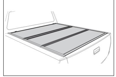
**OPENING COVER:** Lower the tailgate and pull the cable on either side. While pulling on the cable lift the panel up and towards the cab.
