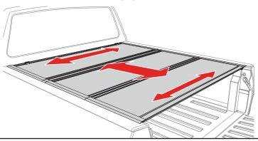
The rear edge of the cover (A) and tailgate seal should rest on top of the tailgate. You are ready to drive with your cover in the closed position.
