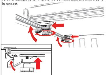
Unfold the cover (A) towards the tailgate. Then confirm each panel is centered side to side and front to back on the truck bed. If adjustments are needed, loosen the cover retainer clamps (D) and shift the cover (A) until positioned correctly. Retighten the cover retainer clamps once the desired fitment is reached. If adjustments to the slam latch are needed, see the directions on the next page.
