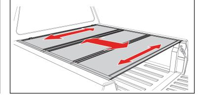
The rear edge of the cover (A) and tailgate seal should rest on top of the tailgate. You are ready to drive with your cover in the closed position.
