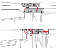
Slide the slots in the 4 bar hinges (attached to the cover) over the posts on the front mounting brackets. Then push the cover forward to lock the hinges to the mounting brackets.
