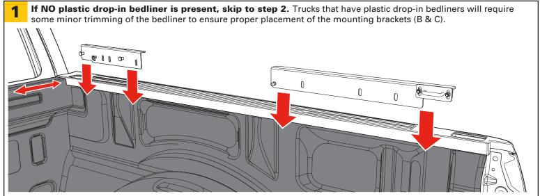
REAR mounting brackets. The rear bracket (B) should be installed on the truck bed rail near the tailgate. To determine the exact location, measure from the back side of the bulkhead to the front edge of the bracket. The specific dimensions for your vehicle can be found on the measurement chart located on the back page of this instruction manual.
