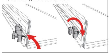
Position the buckle ends (H) with the open side facing the bed cover panel. Use a screwdriver to install the two buckles into the pre-drilled holes on the front header panel with the provided screws (I). DO NOT use a screw gun, securely tighten by hand only.
