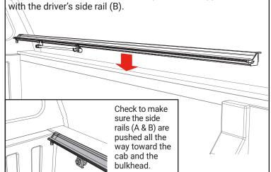
Attach three clamps (G) to the driver side rail (B) to the truck bed. Place the front clamp 6-8 inches from the bulkhead. Place the rear clamp as close to the tailgate as possible. Center the middle clamp accordingly. Clamps should be evenly spaced along the full length of the rail. Loosely tighten with a 1/2" wrench to make sure the clamps engage with the side rail. Repeat on the passenger side rail (A).
