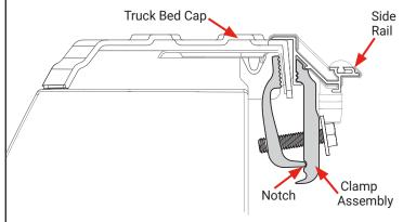
Before placing the cover (C) onto the vehicle, slide two front cover retainer clamps (F) into the track on the underside of the cover (C) near the cab. Confirm the cover retainer clamps fit properly into the cover rail for optimum fit. Repeat on the opposite side of the cover.
