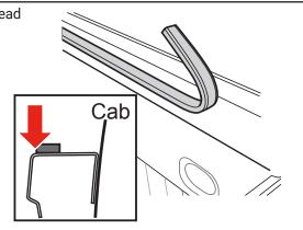
If rubber filler strips (E) were **NOT** included in your kit, skip to step 3. If you received rubber filler strips (E) with the cover (C), clean the rail the same way as you did in step 1. Peel the backing and adhere the filler strips (E), as illustrated, between the truck plastic bed cap and truck metal rail. Place one 6-8 inches from the bulkhead. Place the rear strip as close to the tailgate as possible. Center the middle strip appropriately.
