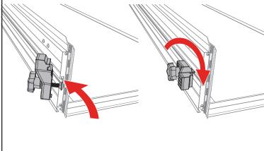
Position the buckle ends (H) with the open side facing the bed cover panel. Use a screwdriver to install the two buckles into the pre-drilled holes on the front header panel with the provided screws (I). **DO NOT use a screw gun, securely tighten by hand only.**
