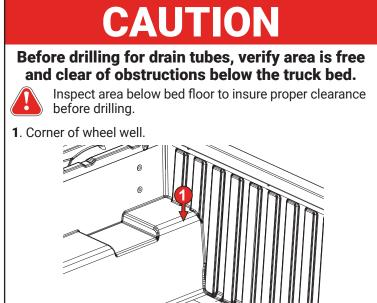
Attach the drain tubes (J) to the front of the side rails (B & C) to allow water to be diverted out of the truck bed via the rail. Drill a 5/8" hole in the top corner of the wheel well as shown in the CAUTION Step (location 1), then run the opposite end of the drain tube through the 5/8" hole.
