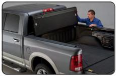
Secure the cover by attaching the prop rods. Remove the prop rod from the j-clip on the cover mounting rail. Attach to the cover by pressing onto the ball stud. To close simply reverse this process.
