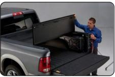
If this is as far as you would like to open the cover, you can secure it in this position. Release the strap from the stowed position by squeezing the tabs. Attach the buckle at the bulkhead, pull the strap to take up the slack and secure the cover.
