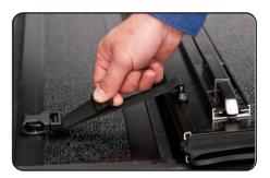
The UnderCover Flex has been outfitted with a very secure latching assembly to allow the truck to be operated with the cover in the fully open position. To open to this position, turn the red handle to the open position and raise the cover.
