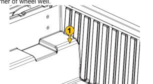
Attach the drain tubes (L) to the front of the side rails (B & C) to allow water to be diverted out of the truck bed via the rail. Drill a 5/8" hole in the top corner of the wheel well as shown in the CAUTION Step (location 1), then run the opposite end of the drain tube through the 5/8" hole.
