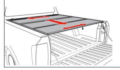
The rear edge of the cover (A) and tailgate seal should rest on top of the tailgate. You are ready to drive with your cover in the closed position.
