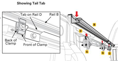
**NOTE:** If the rails are leaning down, have one person stand on the outside of the bed and slightly roll the rails upward while another person slowly snugs the clamps up. If the clamps are tightened too quickly or overtightened, it will cause the rails to lean down.
