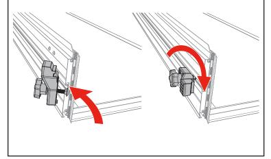
Position the buckle ends (H) with the open side facing the bed cover panel. Use a Phillips screwdriver to install the two buckles into the pre-drilled holes on the front header panel with the provided screws (I). DO NOT use a screw gun, securely tighten by hand only.
