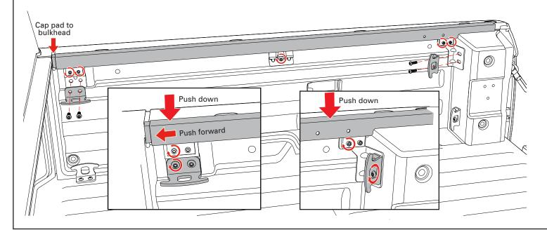
If rubber filler strips (E) were **NOT** included in your kit, skip to step 3. If you received rubber filler strips (E) with the cover (C), clean the rail the same way as you did in step 1. Peel the backing and adhere the filler strips (E), as illustrated, between the truck plastic bed cap and truck metal rail. Place one 6-8 inches from the bulkhead. Place the rear strip as close to the tailgate as possible. Center the middle strip appropriately.
