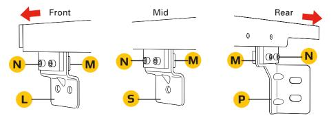
If the rail is not seated properly on the bed cap and a gap is visible between the rail and the truck bed, try the following bracket orientation:
