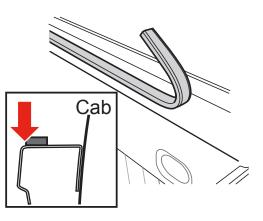
Before placing the cover (C) onto the vehicle, slide two front cover retainer clamps (F) into the track on the underside of the cover (C) near the cab. Confirm the cover retainer clamps fit properly into the cover rail for optimum fit. Repeat on the opposite side of the cover.
