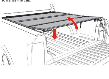
FOLDED UP POSITION: To drive with the cover (C) in the folded up position, use the straps and buckles provided with the cover. Attach the buckle at the bulkhead, then pull the strap to take up the slack and secure the cover.
