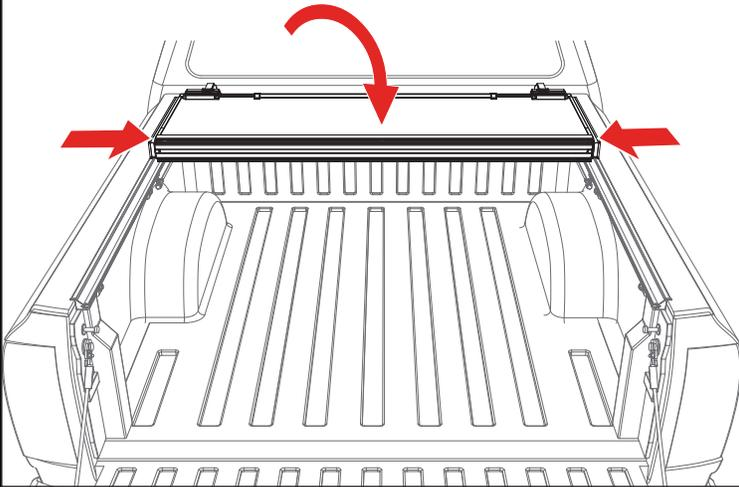
**10** Confirm the retainer clamps (G) are positioned around the side rails (B & C) correctly as shown below. Tighten the retainer clamps by turning them clockwise until the lock washer is secure.
