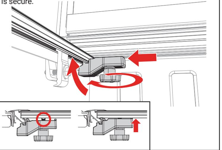
**11** Unfold the cover (A) towards the tailgate. Then confirm each panel is centered side to side and front to back on the truck bed. If adjustments are needed, loosen the cover retainer clamps (G) and shift the cover (A) until positioned correctly. Retighten the cover retainer clamps once the desired fitment is reached. *If adjustments to the slam latch are needed, see the directions on the next page.*
