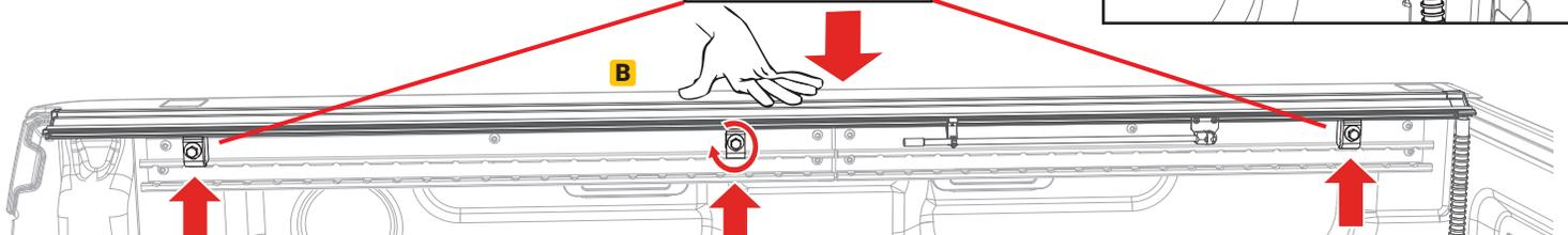
**NOTE:** If the rails are leaning down, have one person stand on the outside of the bed and slightly roll the rails upward while another person slowly snugs the clamps up. If the clamps are tightened too quickly or overtightened, it will cause the rails to lean down.
