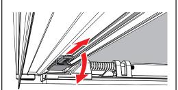
With the tailgate open, pull cord downward on one side to disengage both slam latches from both sides.
