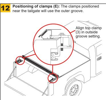
Secure the clamps (E): Roll the cover back to the front. After positioning the clamps correctly and connecting them to the side rails, securely tighten the clamps in position. Ensure that the clamps are tightened sufficiently to hold the side rails firmly in place.
