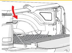
Grasp the tailgate header before releasing the slam latches.
