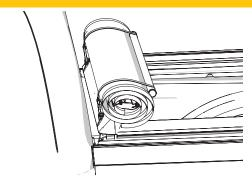
Roll up the cover (C). Do not disengage the hook and loop fasteners before rolling the cover. Always secure the cover at the front with both retainer straps.
