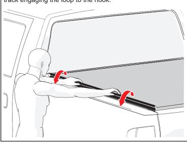
hand to firmly push the loop strip into the hook track. Do this to both driver and passenger sides. You are ready to drive with the cover (C) in the closed position.
