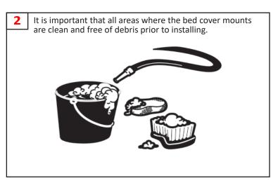
Install the bulkhead weather seal (D) to the truck's front bulkhead: Clean the area where the seal will go with soap and water to remove dirt and debris. Then clean the area with isopropyl alcohol to remove wax or grease and to evaporate any remaining water, allow the surface to dry. Then position the seal and apply pressure to the entire seal to make sure the adhesion is good.
