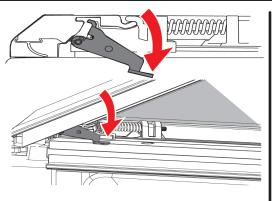
With the tailgate open, press down-ward on one side latch to disengage.
