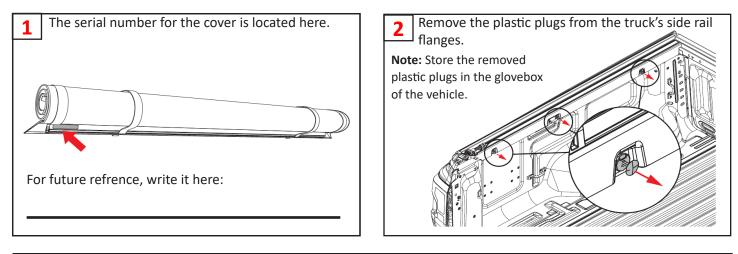
3 Install the bulkhead weather seal, item (G), to the truck's front bulkhead. Clean the area where the seal will go with soap and water to remove dirt and debris. Then clean the area with isopropyl alcohol to remove wax or grease and to evaporate any remaining water, allow the surface to dry. Then position the seal and apply pressure to the entire seal to make sure the adhesion is good.
