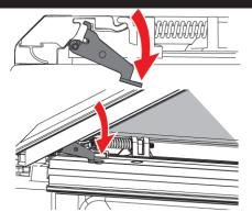
With the tailgate open, press downward on one side latch to disengage.
