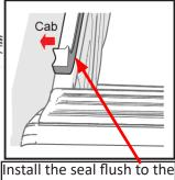
Install the seal flush to the inside face of the truck's bulkhead as shown.
