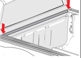
A Remove cab corner seals (E) from the adhesive backing. Place onto both cab ends corner plugs on the driver and passenger side rails (A & B).
