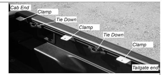
2 Remove tie downs: If tie downs are installed in the cargo rail, remove them for now.
