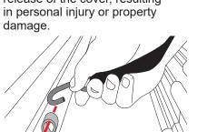
To release strap push tab up. **NOTE:** Ice buildup within hinge sections can occur if cover is stowed in open position. To prevent potential damage, close cover during winter precipitation.
