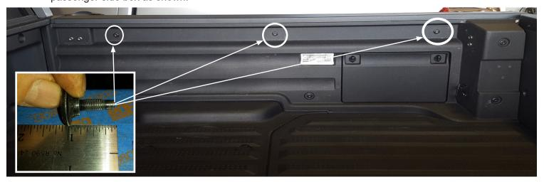
**STEP 2:** Mount brackets on driver and passenger sides using the factory installed M6 Shoulder bolts. Do not fully tighten these bolts, just tighten them finger tight.
