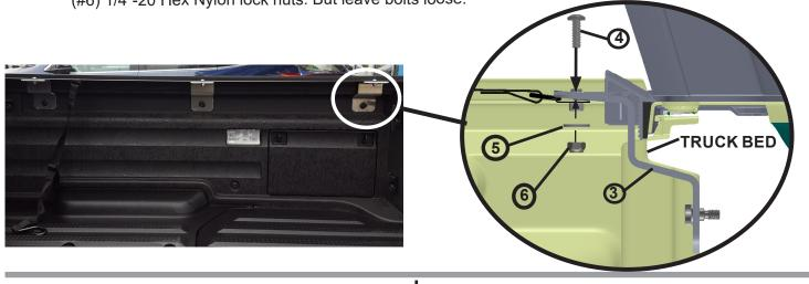
STEP 4: With everything loosely assembled tighten all six M6 Shoulder bolts making the bracket tight to the truck bed, leaving the rails able to move.
