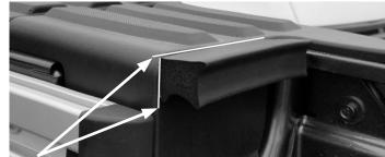
Align seal flush along the top edge of the bed cap and the inner edge as shown.
