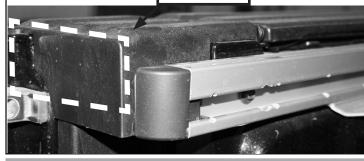
STEP 3. Apply Seal on Driver and Passenger Side as shown below.
