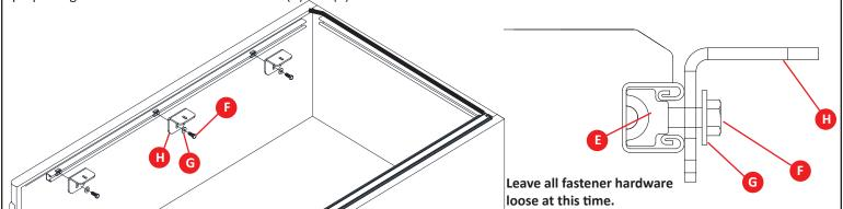
To attach the side rails to the formed brackets, follow these steps:
