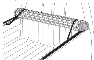
Before driving with the cover open, both straps must be secured to retaining loops. Failure to do so could cause accidental release of the cover, resulting in personal injury or property damage.
