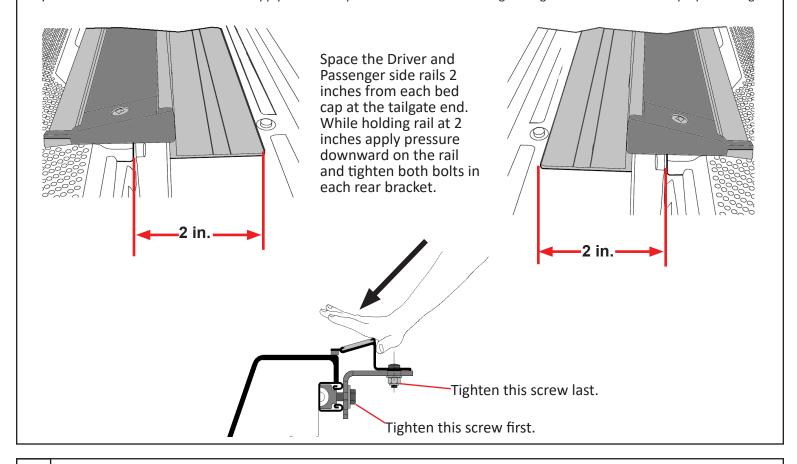
Adjusting the cross car spacing of side rails (A) and (B) at the cab end of the truck bed: At this point, the side rails should already be spaced correctly fore and aft (lengthwise), focusing now on the side-to-side spacing at the cab end.
