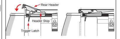
**Preferred method of closure:** Close tailgate, then close cover on top of the tailgate. This method will not work with some truck applications. Use the alternative method instead.
