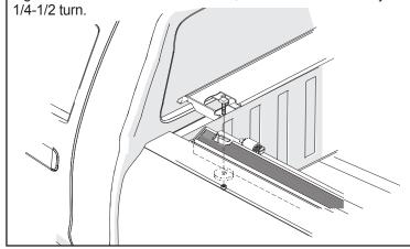
Disengage the retainer hooks from the retainer loops and unroll the cover towards the tailgate.
