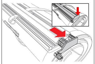
Install the bolts (L) by sliding them into the header as shown below. Do this on both driver and passenger sides. Then reinstall both end plugs.
