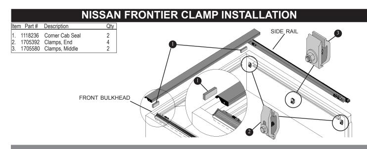
Follow these instructions to install cab corner weather seals and side rail clamps on your 2005 or newer Nissan Frontier pickup. Refer to Owner's Manual for complete installation instructions.
