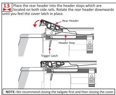
A clicking sound will indicate a correctly installed cover. Next secure the hook and loop fastener along the entire length of both side rails before driving the vehicle. Simply run your hands down both sides of the cover to achieve this. This will prevent wind from lifting the cover and causing possible damage. You are ready to drive with the cover in the closed position.
