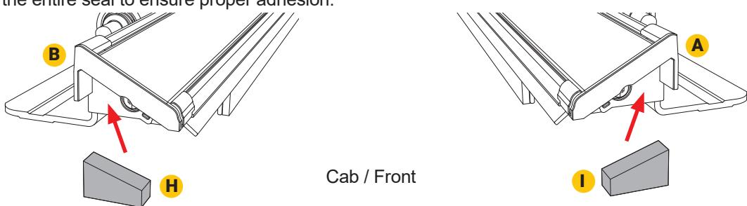
**5** Install the driver side rail (A) using the M6 bolt (D) and the M6 nut (E) to attach the rail to the brackets you installed in step 3b. Repeat on other side with passenger side rail (B) using the same bolt and nut. **Leave loose for now.**
