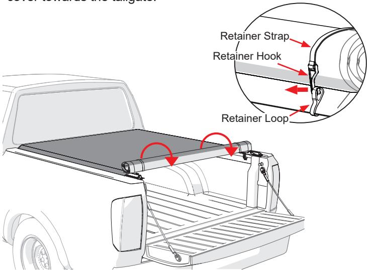
**12** Place the rear header into the header stops which are located on both side rails. Rotate the rear header downwards until you feel the cover latch in place. A clicking sound will indicate a correctly installed cover.
