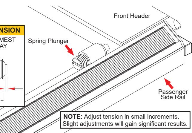
**NOTE:** Adjust tension in small increments. Slight adjustments will gain significant results.
