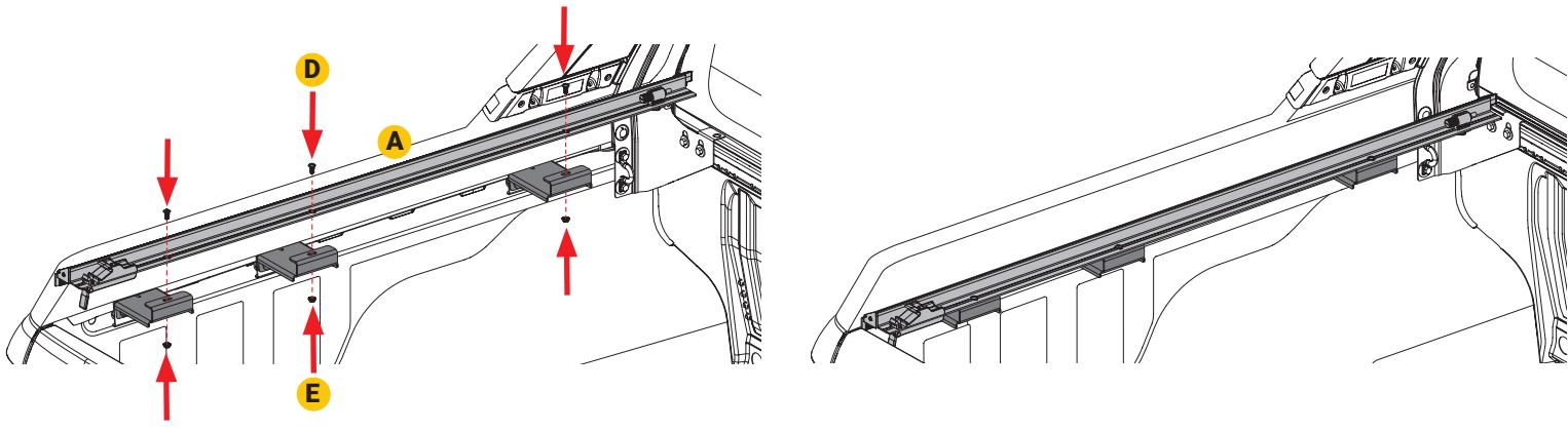
**6** **6a** - Position the driver side rail (A) against the sail while tightening M6 bolts. Side rails should be level with the top of the bulkhead and top of the tailgate. Side rails can be adjusted up or down slightly to create optimal seal on tailgate or bulkhead.
