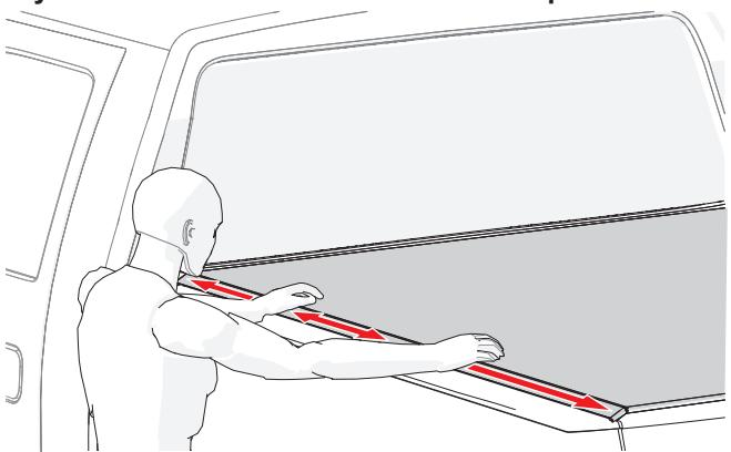
**HOOK AND LOOP MUST ALWAYS BE ADJUSTED AFTER ROLLING COVER CLOSED!**
