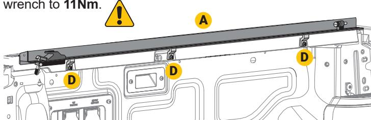
**NOTE:** The use of spring clamps to hold the side rail in place can assist during the installation process.
