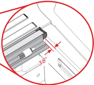
**7** For optimal latching performance and cover fit, the side rails (A & B) should be level with the truck bed caps and not tilted up or down. To fine-tune side rail tilt, you can reposition the clamps (D). To adjust the rail tilt upwards or downwards. Tighten all clamps (D) with a T-30 drive socket or T-handle wrench to **11Nm**.
