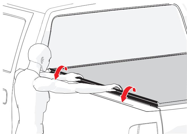
**16** With both sides of the hook and loop engaged, use the palms of your hand to firmly push the loop strip into the hook track. Do this to both driver and passenger sides. **You are ready to drive with the cover in the closed position.**
