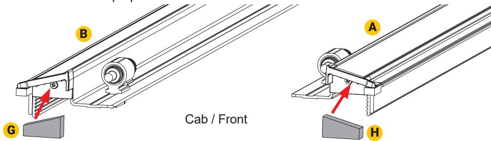
**6** Position the driver side rail (A) to the inside of the truck's bed rail, making sure the flange of the driver side rail fits on top of the bed cap. The front edge of the rails will be 9.5mm back from the bulkhead.
