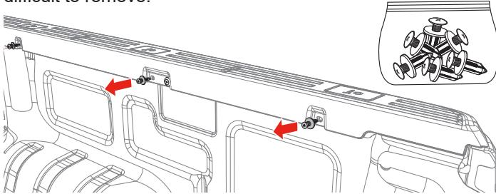
**4** Install the six clamp brackets (D) to the truck box in the locations where you removed the factory plastic clips from in step 3. The lock nut from clamp (D) goes behind the plastic bed cap and sheet metal of the truck. Leave hardware loose at this time.
