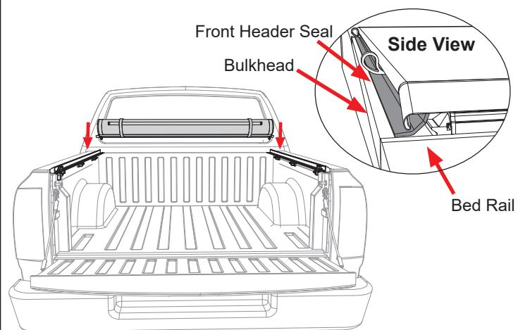
**12** To connect the cover assembly (C) to the side rails (A and B), slide the right and left header guides into the locked position. A clicking sound will indicate a secure attachment.
