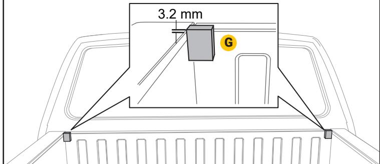
**3** Remove three of the four factory plastic clips as shown below. Unscrew the center first, then pry out the entire clip. These will not be used again unless you permanently remove the bed cover assembly. Caution: Be careful when removing plastic clips. These clips are screwed in and at times from the factory are stripped out making them a bit more difficult to remove.
