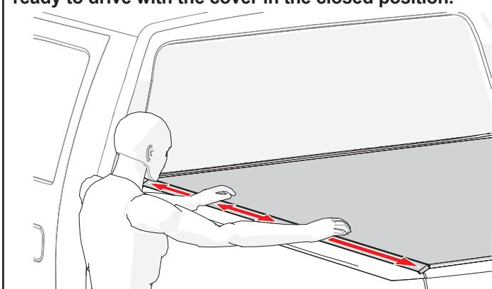
**HOOK AND LOOP MUST ALWAYS BE ADJUSTED AFTER ROLLING COVER CLOSED!**
