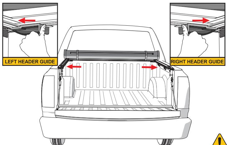
**13** To drive with the cover in the closed position, disengage the retainer hooks from the retainer loops and unroll the cover towards the tailgate.
