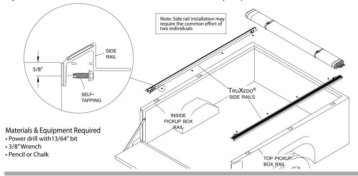
STEP 1: TruXedo® Lo Profile side rails have four prepunched mounting holes. Hold side rails against front of box, keeping offset portion of rail flush with top rail of box. Chalk mark locations of four holes on inside of pickup box, using mounting holes as guides.
