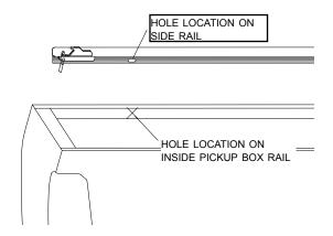
STEP 2: Make sure hole locations are about 5/8" down from top edge of pickup box. Drill 13/64" holes at marked locations.
