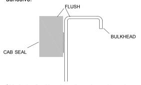
STEP 2: Side Rails: Position side rails against cab weather seal as shown below. See Owner's Manual for complete instructions.
