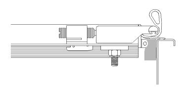
STEP 3: Side Rail Clamps: If your pickup bed does not have Utili-track channels, install three clamps on each side rail as shown in owner's Manual. If your pickup bed does have Utili-track channels, install two clamps on each side rail, locating clamps at each end of Utili-track
