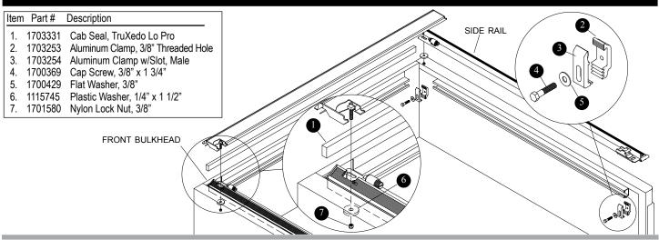
Follow these instructions to install cab weather seal. side rail clamps, and cab header on your 2005 or newer Nissan Frontier pickup. Refer to Owner's Manual for complete installation instructions.
