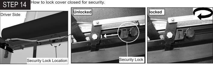
The Deuce cover can be locked while the cover is rolled up or in the open position as shown above.
