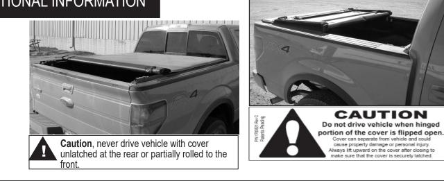
To prevent accidental release of tailgate header, ensure rear header is securely latched to the side rails before driving vehicle.
