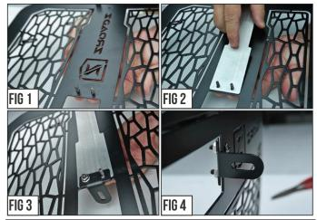
STEP 2 Put into place one of the Bracket Tabs and seucre with provided Hardware as seen in Fig. # 1-4.
