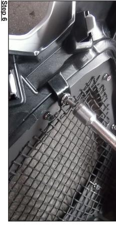
Secure grille studs with the included brackets and locknut's
